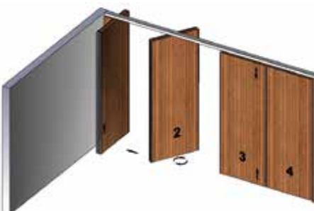
Pic. 9: Example of the panel movement with a single point suspension.
